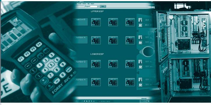
Stock's Forry line was the first to introduce digital controls for electrostatic precipitators over 25 years ago. Forry innovation continues today with our full line of modern voltage controls, rapper controls and T/R sets.
